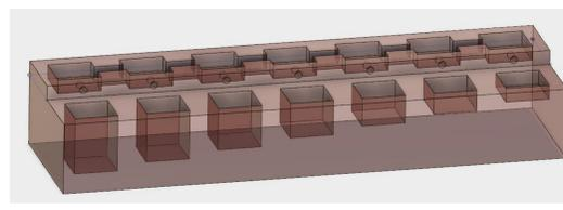
Fig. 4. Top layer contains RNA, dispersed via a channel. Bottom piece has wells with different amounts of water.
