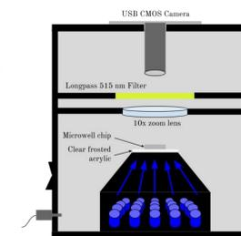
Fig. 6. Imaging Device
