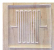
Fig. 3. Acrylic chip with channels etched in.
