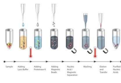
Fig. 1: RNA Extraction with Magnetic NanoBead Technology
