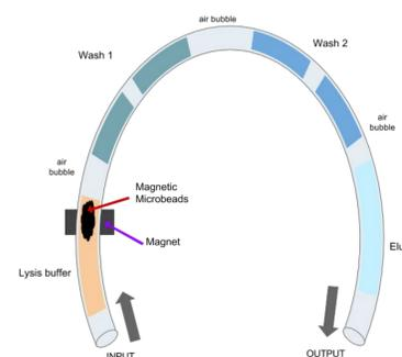
Fig. 2: Microchannel Design for Reagent Delivery
